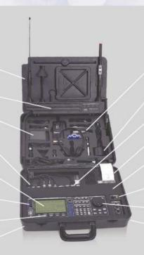
RF LOCATOR PROBE FOR LOCATING TRANSMITTERS
