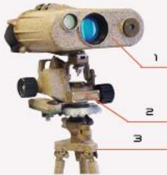
1 - RANGEFINDER; 2 - ANGULAR INSTRUMENT 3 - TRIPOD
