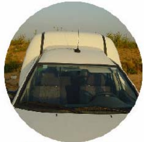
Vehicle mount magnetic base antenna
