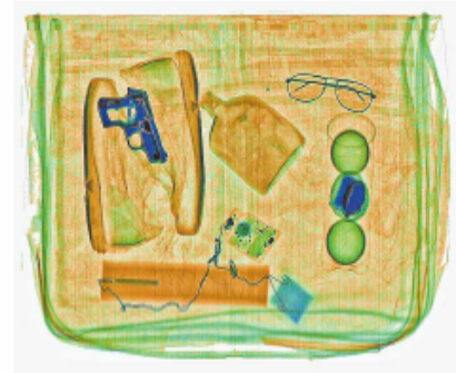
RealClear® reveals components of a gun, knife and bomb in real time, without lags and delays.
